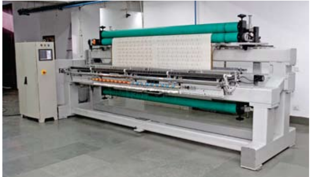
The world's first Vertical Computerized Embroidery Machine (VEM), with 150 inches in length it can use 3 widths of 48 inches long fabrics
